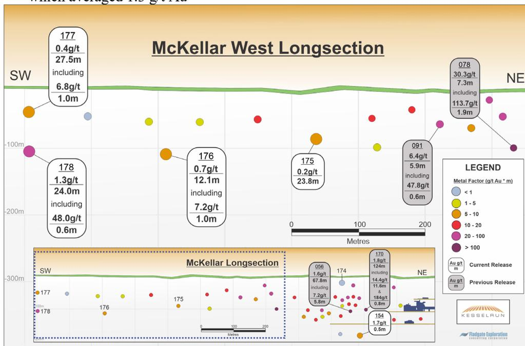
Figure 2. Schematic Long Section – McKellar Zone
